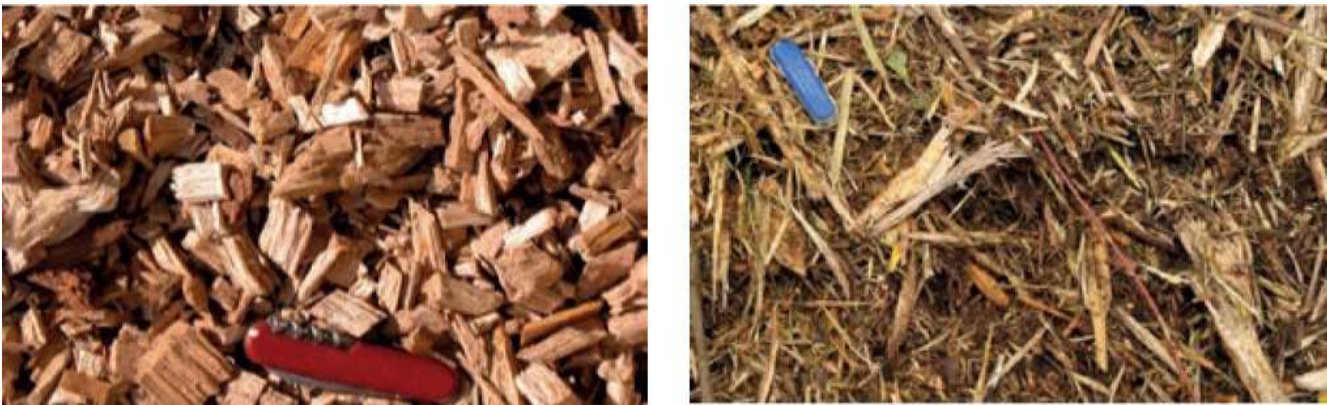
Figure-4-Wood chips (left) cannot be efficiently decomposed by compost microorganisms, whereas defibered wood (right) can. The use of defibered wood results in a better structure within the windrows and allows for a better aeration.
